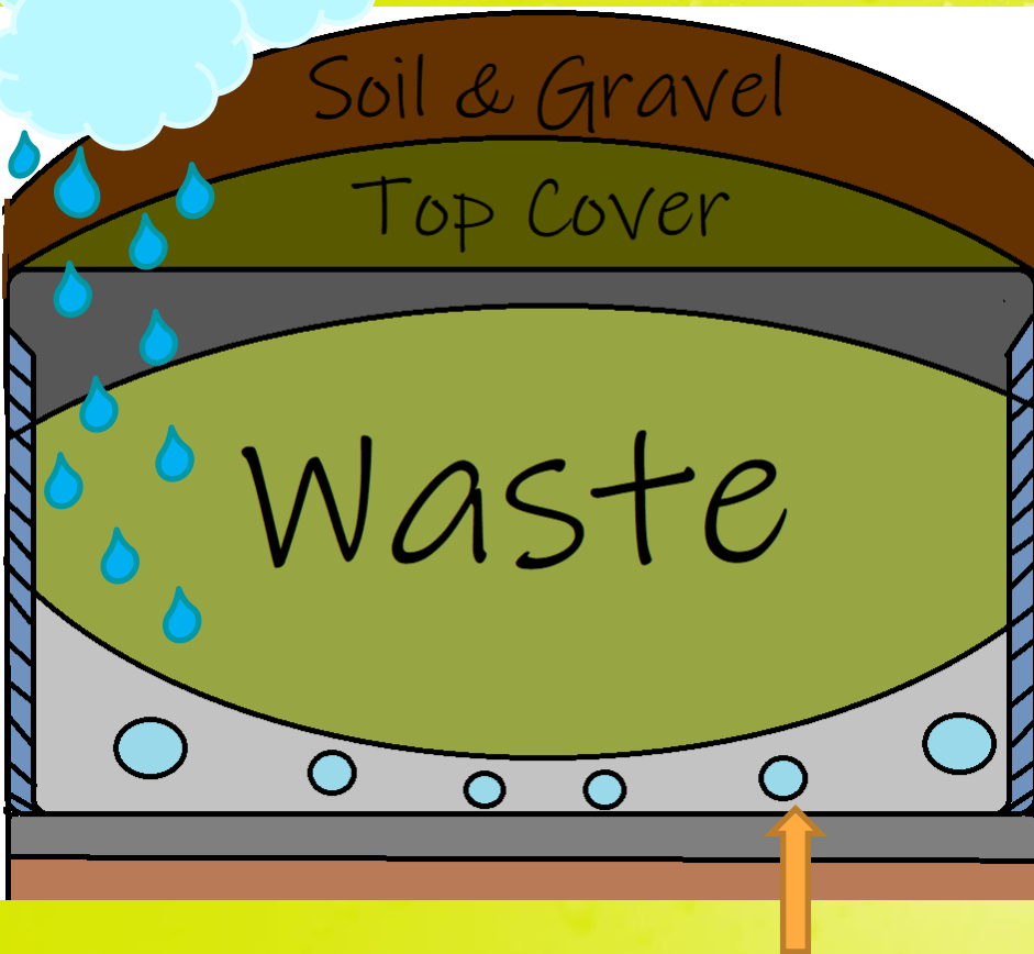
Leachate collection piping networks
